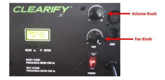
Priming the Pump using Volume and Fan knobs.
